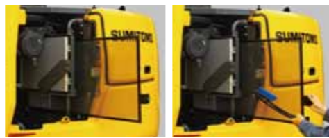
*) Blockage of the front face protection net for radiator can cause malfunctions. Clean the net regularly.
