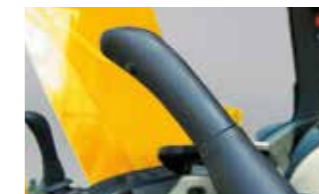
Radio mute switch (left lever)
