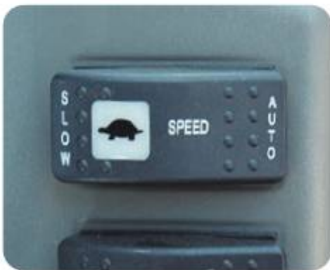
Travel speed mode switch
