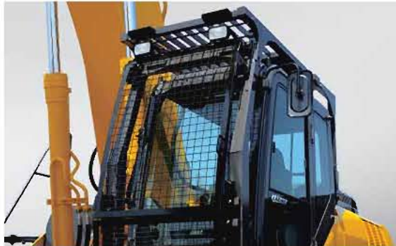
Cab-top light/Front mesh guard/ Head guard(FOPS level 2)
