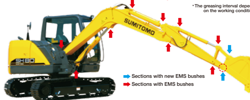
A Solid lubricant B Dust seal Plated pin Special bushing High strength brass A solid lubricant embedded in high strength brass forms a layer on the bushing surface to prevent contact between metals, maintaining an excellent lubricated state to reduce abrasion of joints. ② The surface of the pin is plated to increase surface hardness and improve wear resistance.
