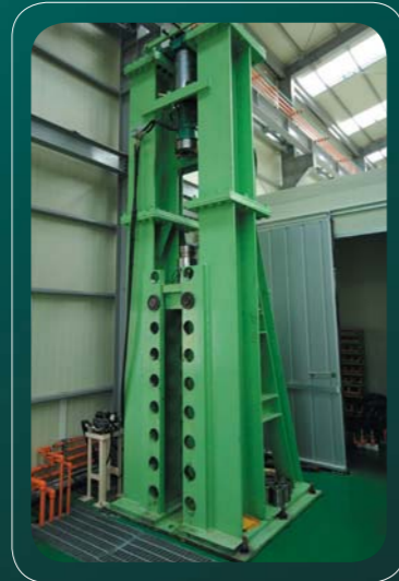
Static calibration test stand for correct measurement
