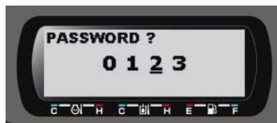
Anti-theft alarm system
